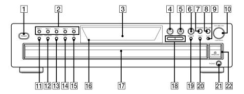
CHECK 20 (11, 12) CLEAR 9 (11, 12) DISC 1–5 2 (7, 8, 11) DISC sompartment 17 (7) DISC SKIP 8 (7, 10, 12) Display 3 (9) EX-CHANGE 7 (10, 13) FADER 13 (12) PEAK SEARCH 12 (13)
